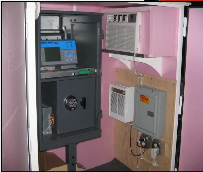
The Mini ATM Kiosk is completely finished inside with 2" rigid foam insulation and sealed against moisture. The 30 amp electrical panel provides separate circuits for the ATM and heating /AC units. The entire kiosk is built of 2" tube steel floors and walls with 14 gauge steel body.
